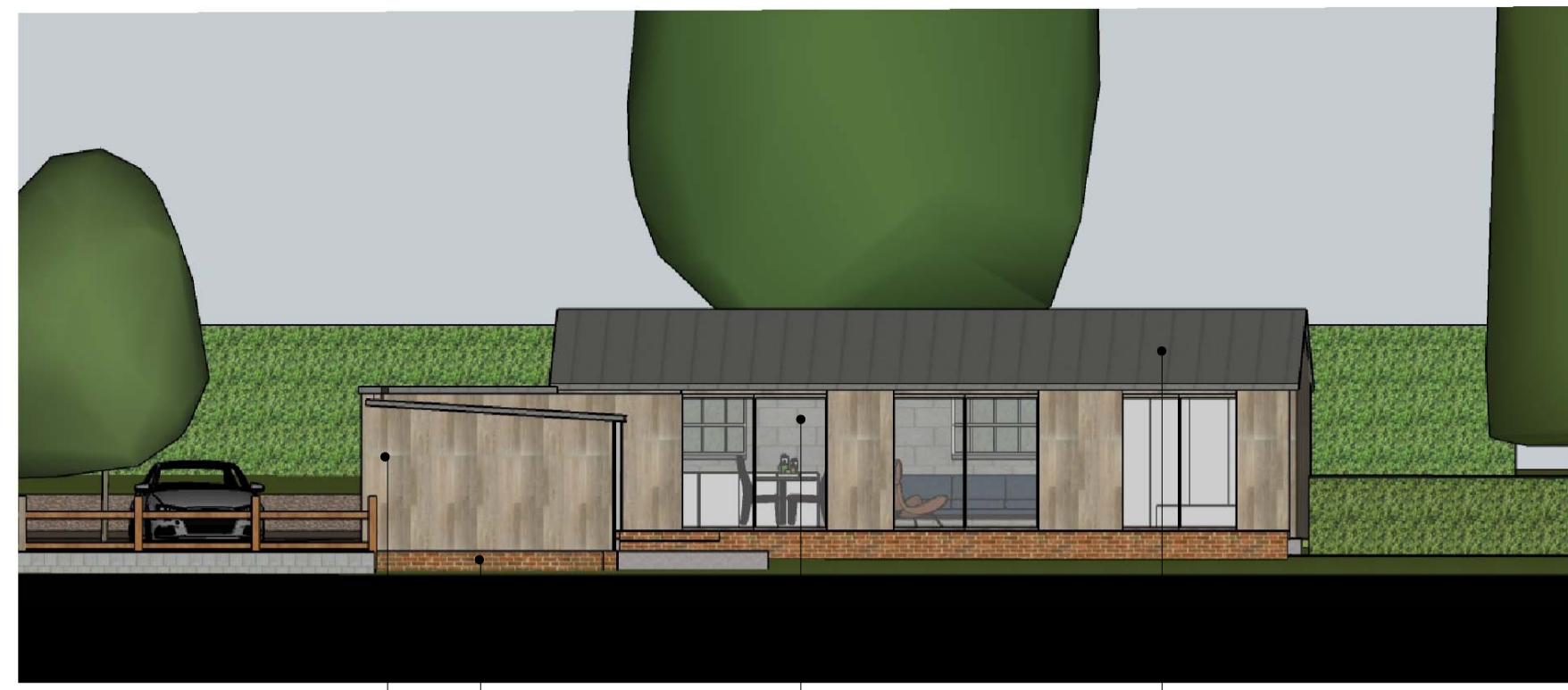
01 170A_1102 WEST ELEVATION LARCH CLADDING EXISTING BRICK FOUNDATION TIMBER DOUBLE GLAZED SLIDING DOORS ZINC ROOF
