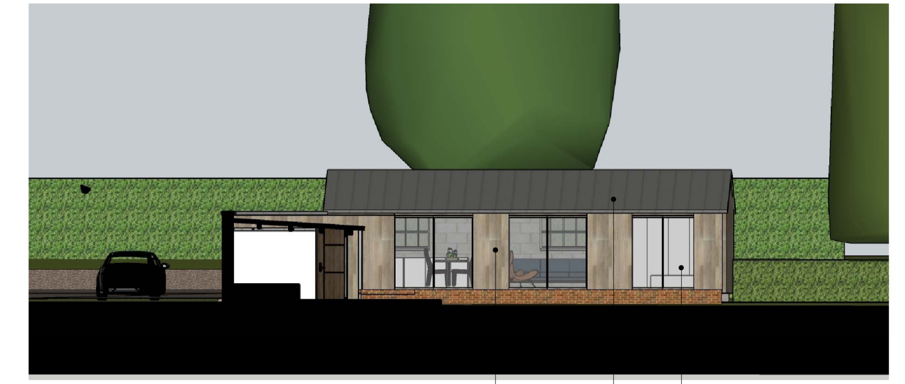
03 170A_1102 SECTION AA LARCH CLADDING ZINC ROOF TIMBER DOUBLE GLAZED SLIDING DOORS
