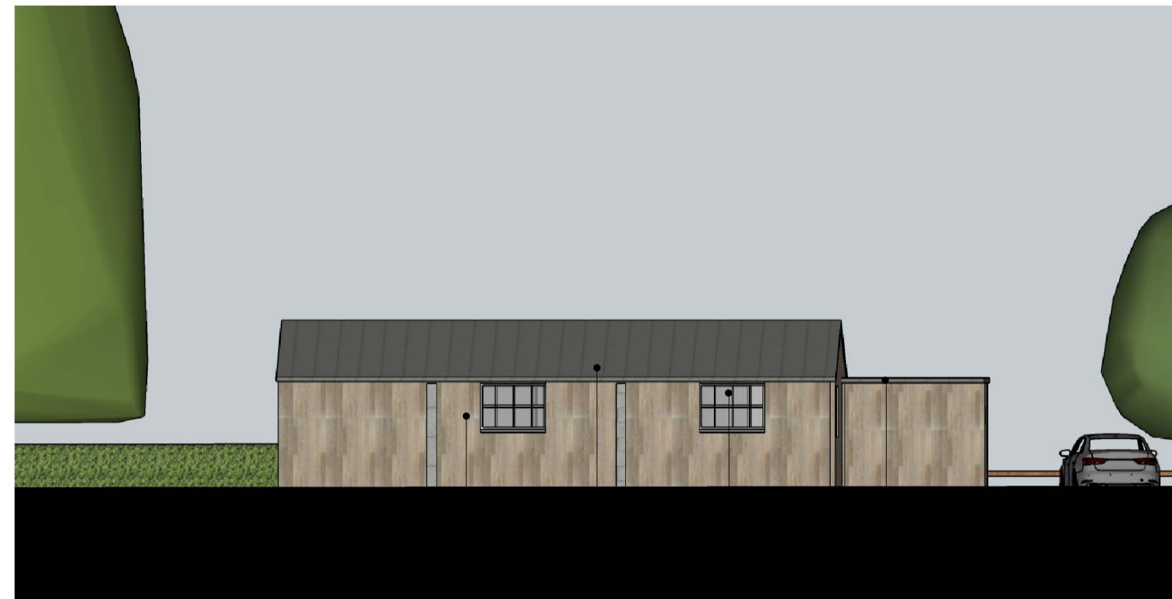
04 170A_1102 EAST ELEVATION LARCH CLADDING ZINC ROOF TIMBER DOUBLE GLAZED WINDOWS ZINC CANOPY
