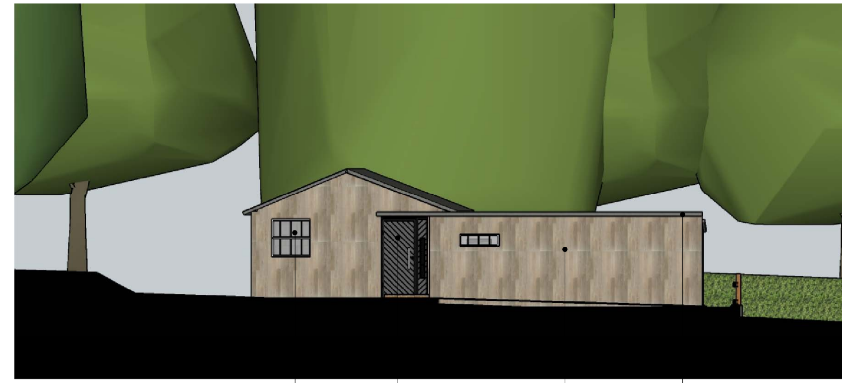
02 170A_1102 NORTH ELEVATION TIMBER DOUBLE GLAZED WINDOWS TIMBER FRONT DOOR LARCH CLADDING ZINC ROOF
