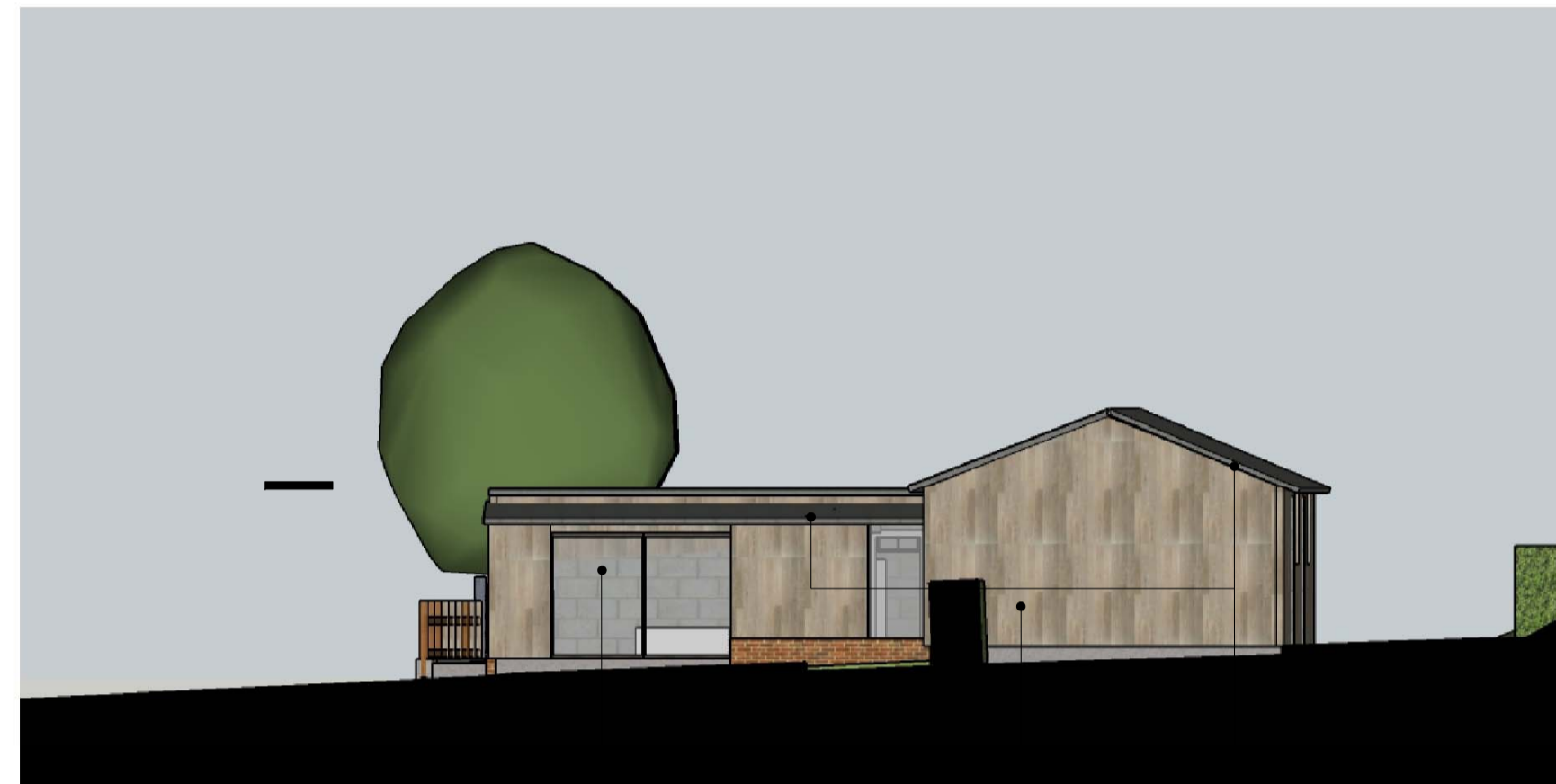
05 170A_1102 SOUTH ELEVATION TIMBER DOUBLE GLAZED SLIDING DOORS LARCH CLADDING ZINC ROOF
